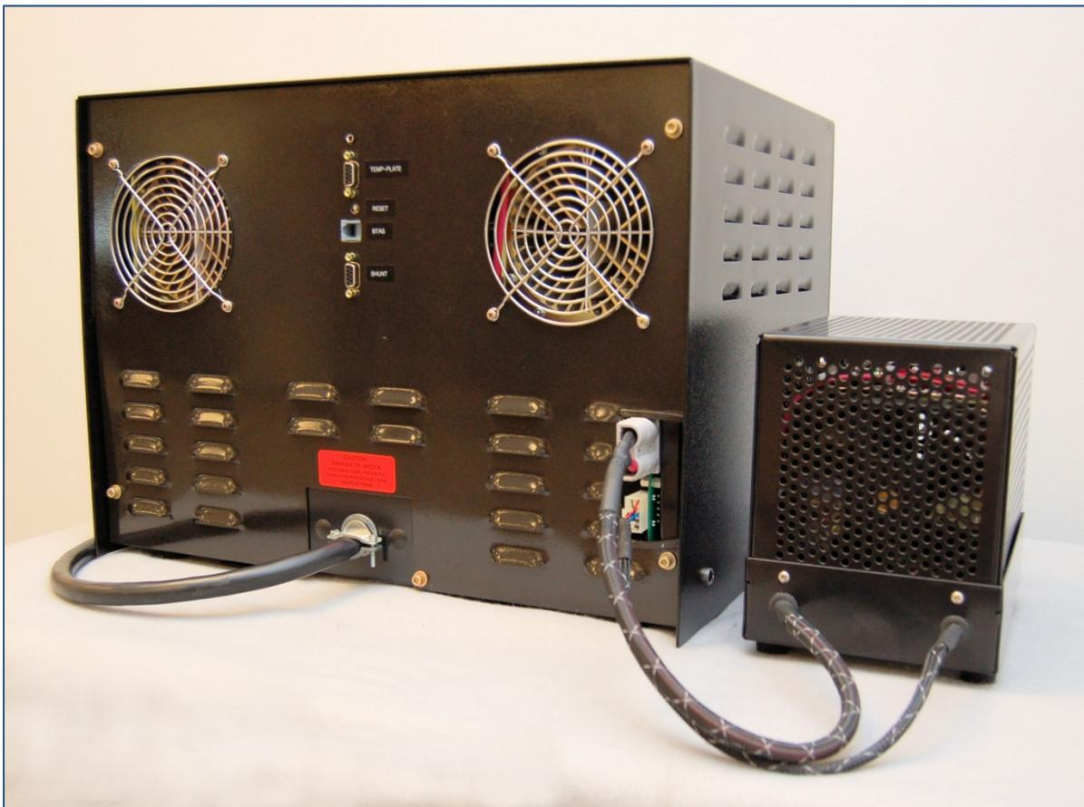
Figure 3 – Connecting the EXD Module to the Charger-Analyzer
