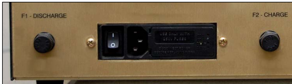
Figure 12 - Power Entry Block and Fuses
